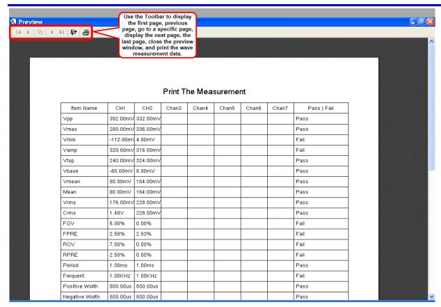
Click the **Print** button on the toolbar to print the waveform measurements.
