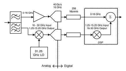
**Figure 1:** Block diagram of Digital Bandwidth Interleave (DBI) technology as used in a WaveMaster 830Zi oscilloscope. In addition to doubling the bandwidth, it also doubles the memory and sampling rate.
