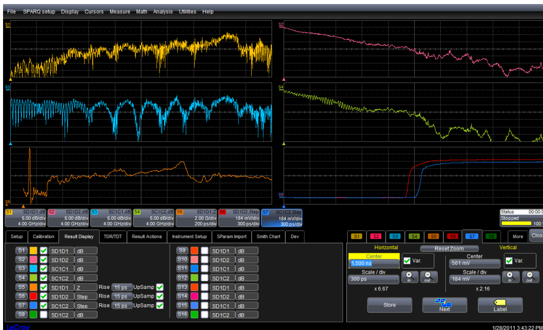
Figure 6: SPARQ application displaying mixed-mode S-parameters and associated time-domain responses.
