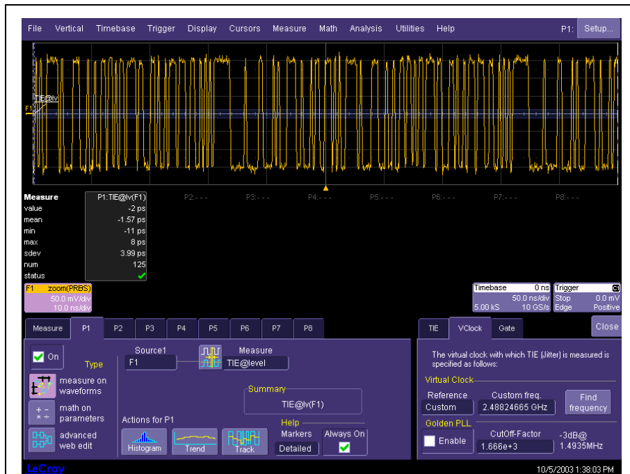
Figure 1 The Virtual Clock tab of the TIE@lv parameter is used to identify the data rate of the pseudo-random bit stream.
