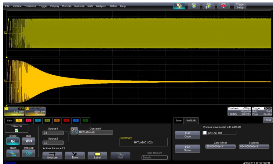
Figure 1: The response of a MATLAB based 2 pole Butterworth filter (lower trace) to a swept sine input (upper trace).
